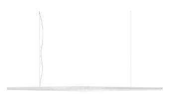
Suspension lighting fixture for interiors, with direct light emission. Machined aluminium structure in white or black polyacrylic paint. Anodized extruded aluminium heat sink. Extruded polycarbonate diffuser with opaline finish. Suspension kit with griplocks and 2m (78,7") long steel cables. 2,3m (90,6") long power cable in transparent PVC. Power canopy with galvanized sheet metal ceiling bracket and pickled sheet metal covering in white or black polyacrylic paint.
